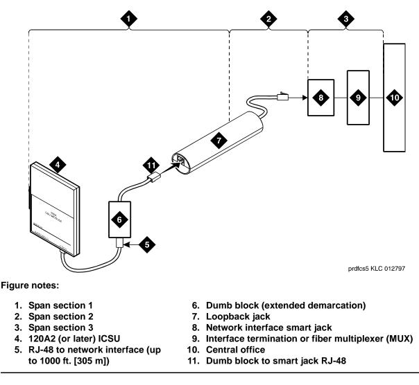
Figure 104: Network interface at extended demarcation point (smart jack accessible) for a 120A2 (or later) ICSU
